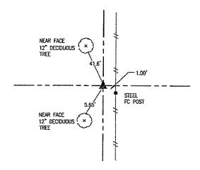
AUGUST 1942 WPA SURVEYORS SET CONCRETE MONUMENT OVER TILE AND PLACED 18" X 14" X 3" SANDSTONE OVER C.M.
